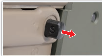
Safety Mode The gun will not fire.
