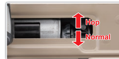
Turn the adjustment dial to adjust hop-up.
