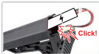
Connect battery until it clicks into place.
