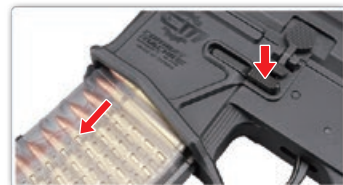
Remove the magazine.
