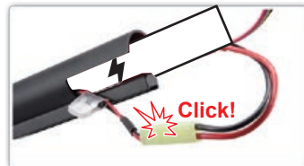
Connect battery until it clicks into place.
