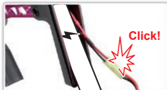
Connect battery until it clicks into place.
