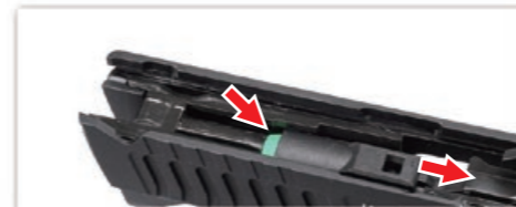
Spray silicone oil on rubber parts.
