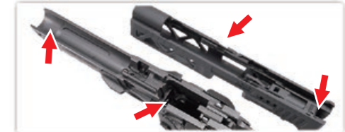
Apply silicone oil for lubrication.
