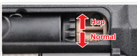
Turn the adjustment dial to adjust hop-up.
