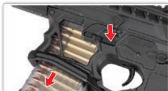
Remove the magazine.
