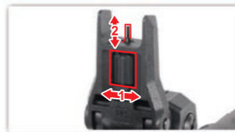
Elevation knob (up / down adjustment).
