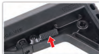
Press the stock release lever to unlock.
