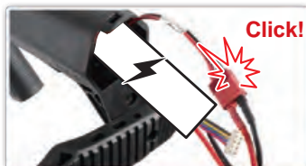
Connect battery until it clicks into place.
