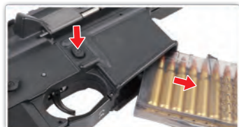
Remove the magazine.
