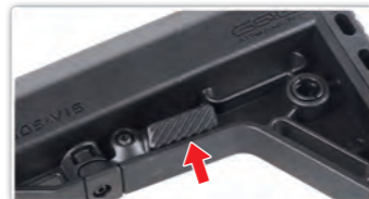
Press the stock release lever to unlock.
