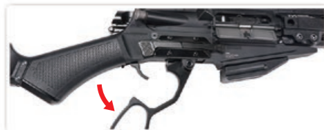
Swing the finger-lever forward will take the bolt back and open the port cover.
