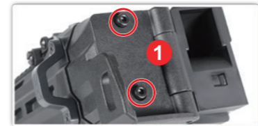
Use 6mm Allen key to remove 2 hex screws on the hinge.
