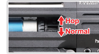
Turn the adjustment dial to adjust hop-up
