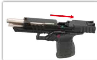
Hold the slide backward as shown.
