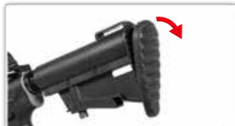
Remove butt stock rubber pad.
