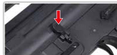
Rotate the Bolt release lever to release the bolt catch.
