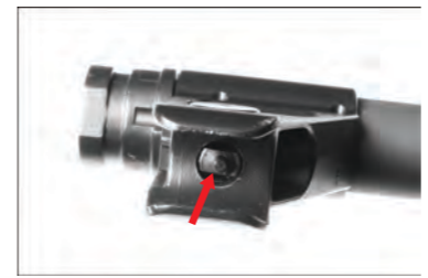
Insert the front sight adjustment tool into the front sight block.
