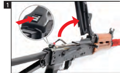
1 Push the cover release button. 2 Remove or lift up the dust cover.
