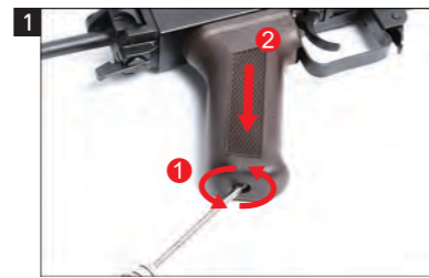
1 Unscrew the fixing screw on the bottom of the grip and remove the grip.
