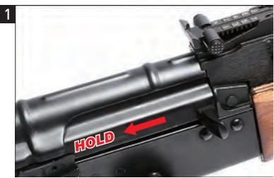
1 Pull the handle in the direction shown to open the bolt.
