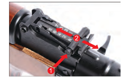
Press the button and slide forward or backward for adjustment.
