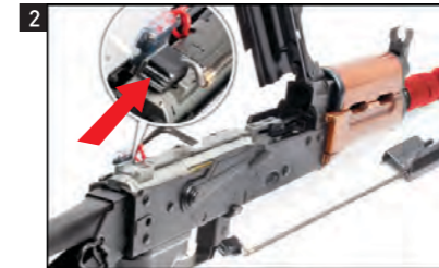
2 Push the rear-end of the spring guide to remove the bolt set.
