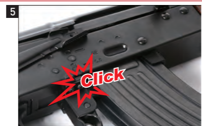
5 Make sure the magazine is securely inserted into the receiver until it clicks.
