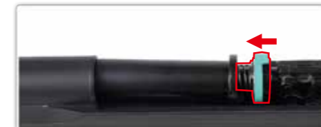
Push the spring rod against plug.
