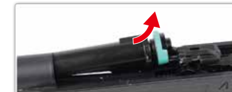
Remove the spring plug and the guide rod.
