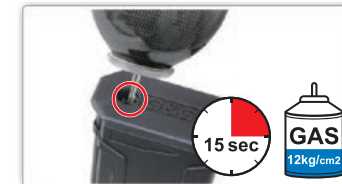
Fill gas through the valve at the bottom of the magazine.
