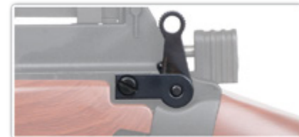
Bolt Lock(Before chambered) Bolt can't be pulled.
