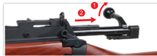
Bolt Lock(Before chambered) Bolt can't be pulled.
