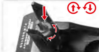
Press the button to adjust front sight up-down. Turning clockwise : Raises the impact point. Turning counterclockwise : Lowers the impact point.
