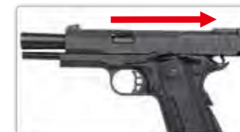
Pull the slide backwards then release.
