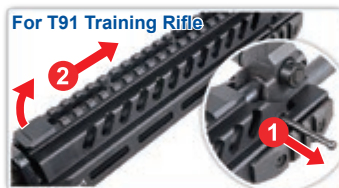
For T91 Training Rifle 1. Pull out the upper rail pin. 2. Push the upper rail forward and pull up from the back of the upper rail to remove.
