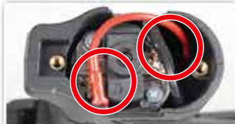
No operation. Check the wire set contact on the motor.
