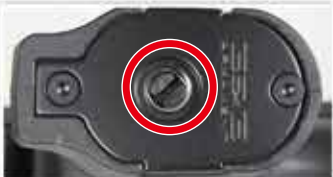
Adjust screw when the gear noise becomes shrilly. Use a screwdriver to adjust the screw at the bottom of the grip.
