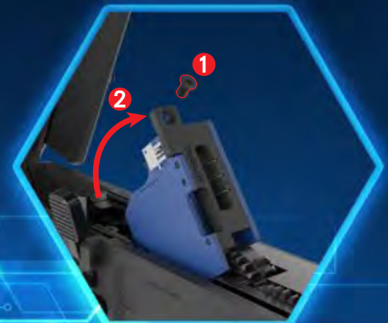
Modular electronic board for easy replacement
