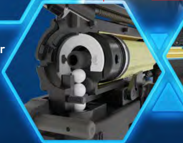
Power-cut off when chamber is empty
