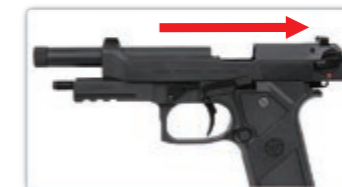
Pull the slide backwards then release.
