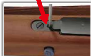
Use an hex screwdriver to loosen the screw locking the hopup dial.
