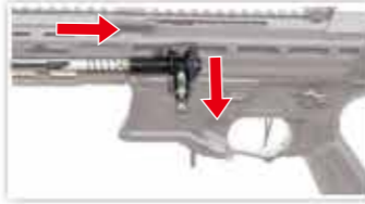
Be sure to have the rod facing down and reaching to the end. Remove clogged pellets.
