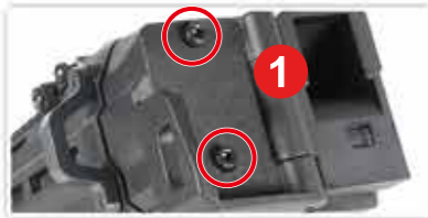
1. Use 6mm Allen key to remove 2 hex screws on the hinge.
