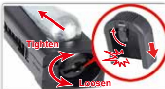
Tab on the rear of the magazine bottom plate then flip out the hex key. Use the hex key to loosen the cartridge tray at the bottom. Install the CO2 cartridge into the magazine and tighten up the tray.
