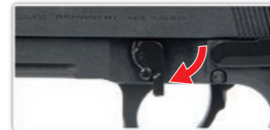
Rotate the latch clockwise until it stops.
