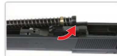
Carefully swing out the recoil spring guide rod and slowly pull it out.
