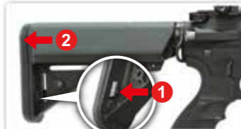
1. Push the butt plate lock (both side). 2. Pull out the butt plate.
