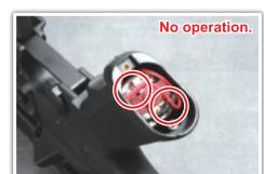
Check the wire set contact with motor.
