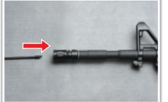
Return the hop up dial to normal position Be sure to have the rod facing down and insert the cleaning rod from the lead edge of the inner barrel.
