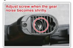
Use a screwdriver to adjust the screw at the bottom of the grip.
