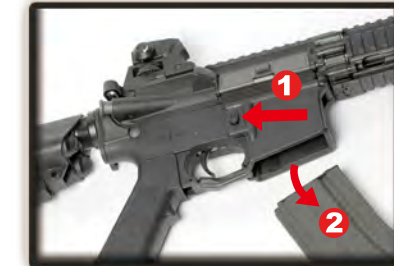
Remove the magazine.
