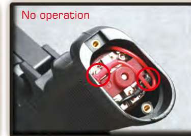
Check the wire set contact with motor.
