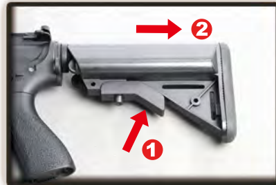
Press the stock release lever to unlock.
