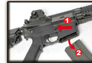
Remove the magazine.
