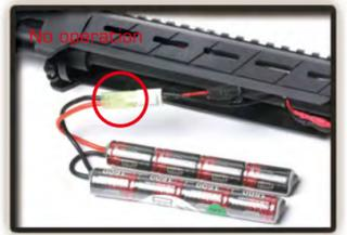
No operation. Make sure the battery is fully charged.
