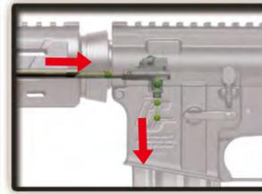
Be sure to have the rod facing down and reaching to the end. Remove clogged pellets.
