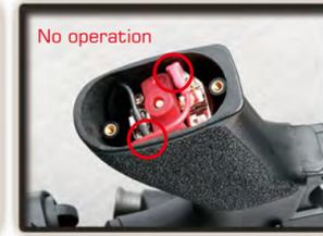
No operation. Check the wire set contact on the motor.
