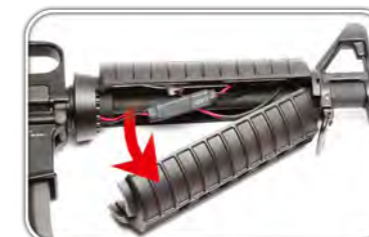
Remove the lower handguard.
