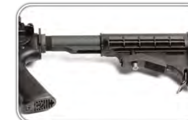
Adjust the position of the stock. (6 positions)
