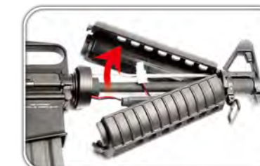
Remove the upper handguard.
