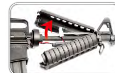
Remove the upper handguard.
