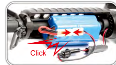
Set the battery beside the outer barrel. Connect the battery plug with the connector until you hear a 'click'.
