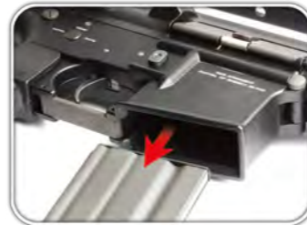
Pull the magazine out of the receiver.
