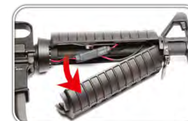
Remove the lower handguard.
