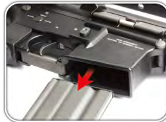
Pull the magazine out of the receiver.
