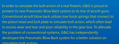
This new technology utilizes compressed air to move the bolt, which enables the action without adding extra stress to the gear box.
