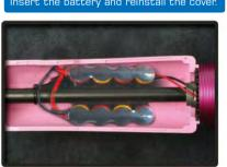
nsert the battery and reinstall the cov
