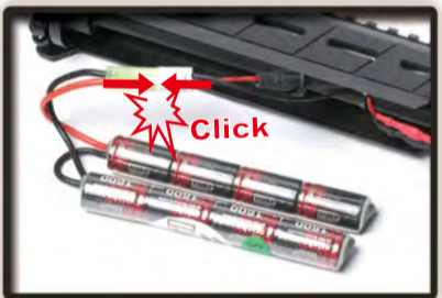
Connect the battery with the connector until it clicks.
