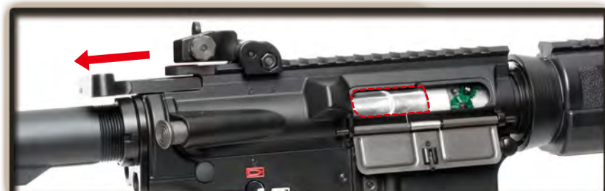
Pulling the charging handle will take the bolt back and open the port cover.
