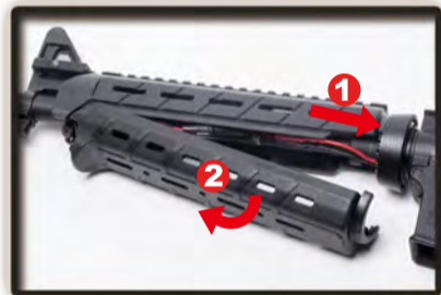
1. Pull and hold down the delta ring. 2. Remove the lower handguard.
