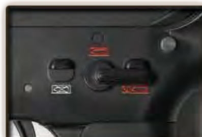
SAFETY ON Trigger will be locked.
