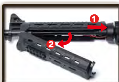
1. Pull the delta ring and hold. 2. Remove the lower handguard.
