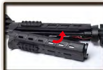
Reinstall the lower handguard.
