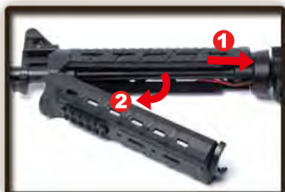
1. Pull the delta ring and hold. 2. Remove the lower handguard.
