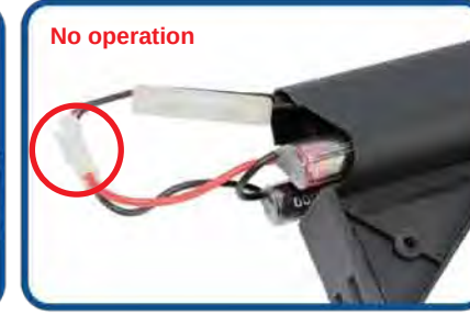
Check the battery and connector.
