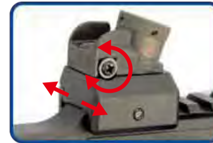
Windage Adjustment (left / right adjustment)
