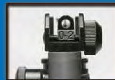
COMMON SHOOTING Used for full automatic firing.
