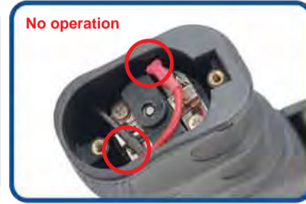
Check the wire set contact with motor.
