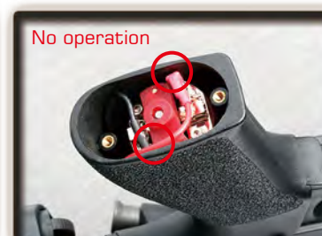
Check the wire set contact with motor.
