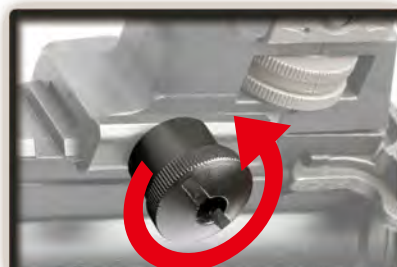
Turn the knobs counterclockwise to disassemble the rear sight.
