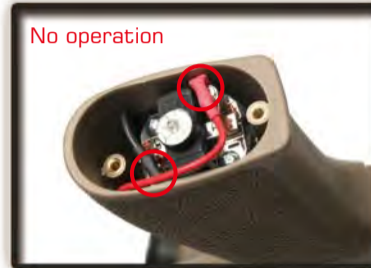
No operation. Check the wire set contact with motor.
