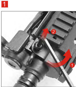
Disassemble the R.A.S. locking screw.
