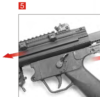
Pull the lower receiver out.
