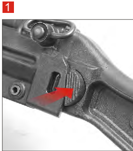
Press the buttstock locking button.
