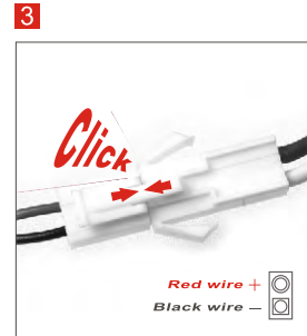
Connect battery plug with the connector.
