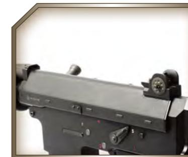
Pull up the lock pin to release the scope mount and take off.
