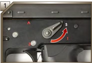
Turn the selector to the Safety position. The magazine should be removed before.
