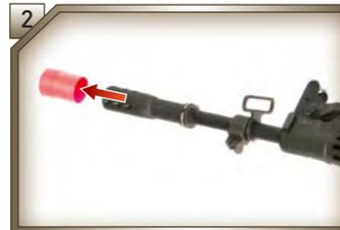
2 Remove the protective cap only when you are ready for firing the gun.
