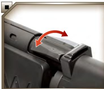
Turn the gas valve to fire rifle grenades. (Simulation)
